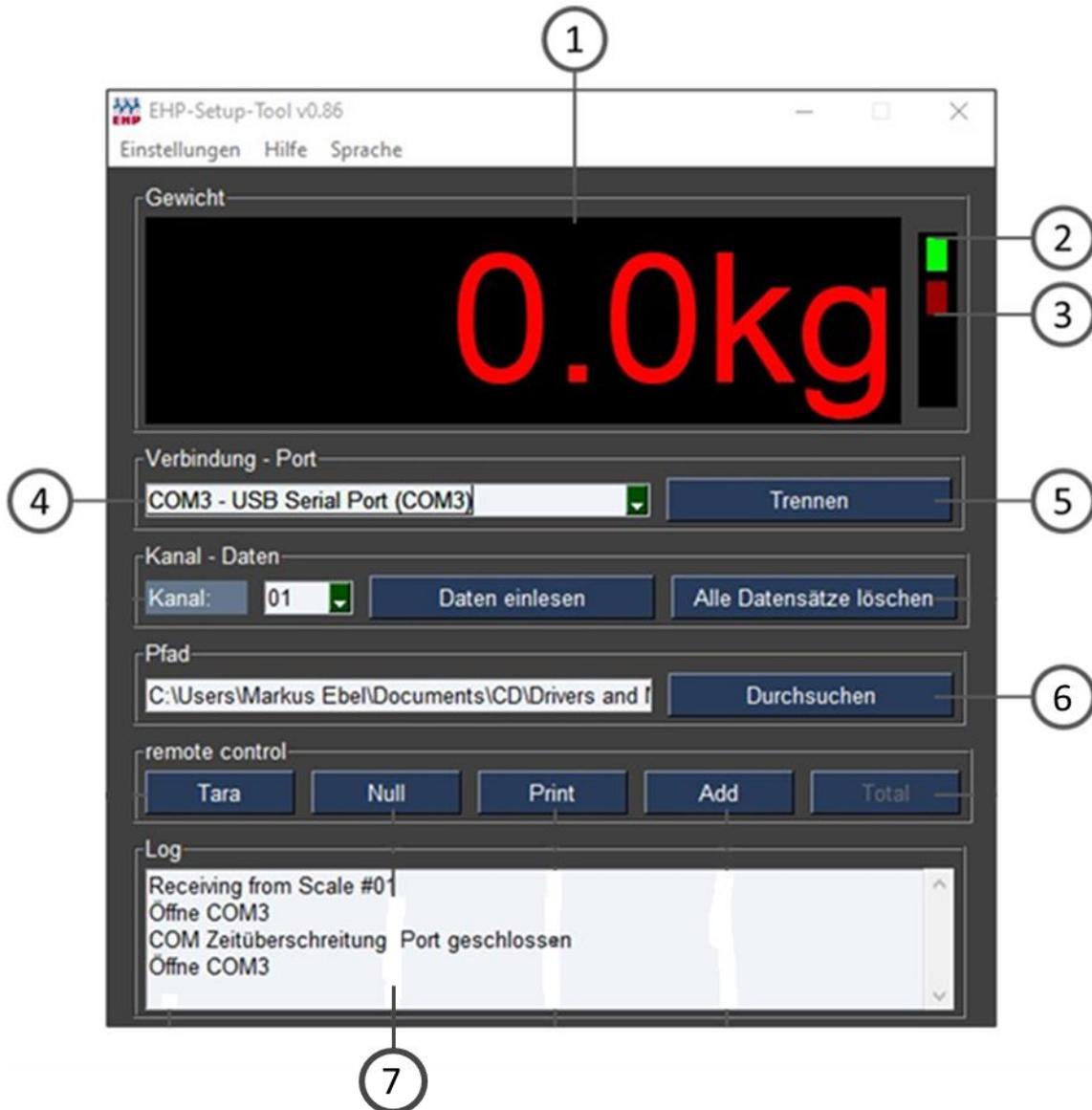
Figure 6- EHP Setup Tool
