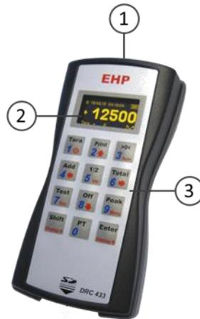
The DRC 433 is equipped with an infrared transmitter, USB port and a charging socket on the top (1). The OLED display (2) and the input keypad (3) are located on the front.
