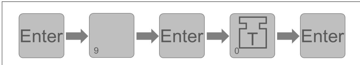
The canal search is indicated by blinking of the transmitter LED. As soon as the scale reacts to the signal of the remote control press ENTER again.
