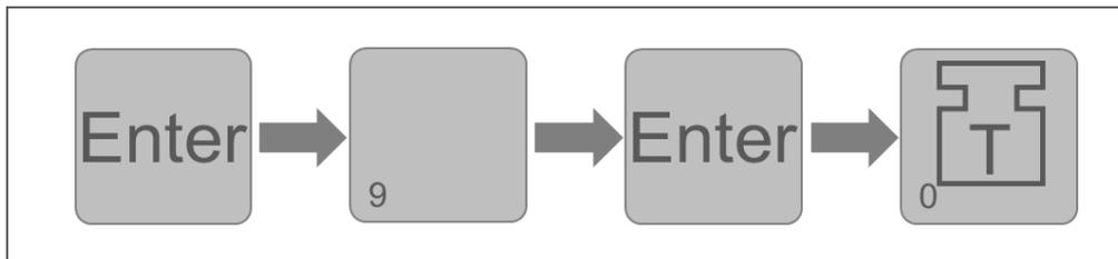
The red LED above the SHIFT key will then light up for 5 seconds, which visualises that you are in the setup menu. During this time the remote control number can be changed.
